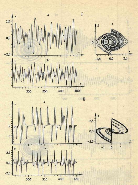
Fig. 9. Time series of the coordinate (a) and velocity (b) and phase portrait (c) of the irregular motion in the system of Fig. 1 at (I)  $\beta=0.1$  and  $F_0=40$  and (II)  $\beta=0.5$  and  $F_0=100$  and the same values for the rest parameters, as for Fig. 2;  $x_0=1.05$
