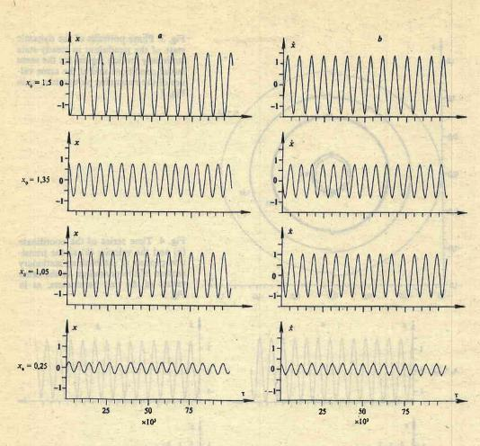
Fig. 2. Time series of the coordinates x(a) and the velocity  $\dot{x}(b)$  in steady-state stationary regime of motion of the pendulum at the following initial conditions:  $x_0=1,5, 1,35, 1,05$  and 0,25. The values of the rest unchanging parameters are:  $y_0=0$ ,  $F_0=2$ , v=51,  $\beta=0,01$ , d=0,025
